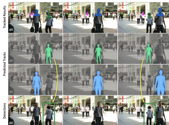
Figure 1. Tracking people by predicting and matching in 3D. The top row shows our tracking results at three different frames. The results are visualized by a colored head-mask for unique identities. The second and third rows show renderings of the 3D states of the two people in their associated tracklets. The bottom row shows the bottom-up detections in each image frame which, after being lifted to 3D, will be matched with the 3D predictions of each tracklet in the corresponding frame. Note how in the middle frame of second row, the 3D representation of the person persists even though they are occluded in the image. Readers are encouraged to watch the videos at the project website .
