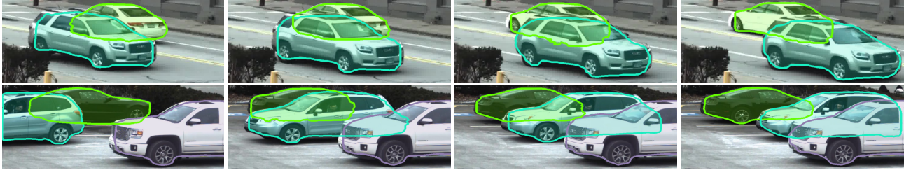
Figure 9. Accurate amodal segmentation of vehicles during occlusion while passing each other (Top) or when a vehicle is parking. Our method is able to provide consistent segmentation and detection of all the vehicles in severe occlusions and motions. This can lead to a drastic improvement in tracking objects with occlusions.
