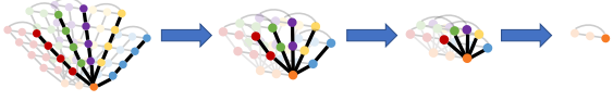
Figure 2. Hierarchical graph structure in the encoding process of UGCN. The spatial edges represent the physical connection of joints. The cross-view edges connect the same joints between any two different views. For easy illustration, we only plot a part of the cross-view edges.
