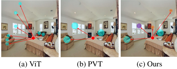
Figure 2. Comparison of different attention mechanisms in Vision Transformer (ViT), Pyramid Vision Transformer (PVT), and our SSA with the same feature map size. The number of circles represents the number of tokens involved in the self-attention computation, and reflects the computation cost. The size of the circle indicates the receptive field size of the corresponding token. Unlike ViT and PVT, our method adaptively merges circles on large objects for enhancing computation efficiency, and accounts for objects of different scales simultaneously, e.g. , cyan for large sofa, purple for middle size window and orange for small size fan and bottle.
