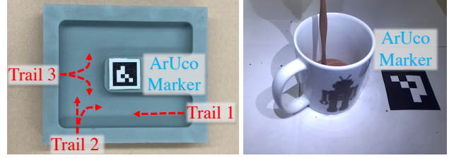
Figure 4. The left figure shows a top down view of the silicon cavity used for the Endoscopic Liquid dataset, and the liquid is injected with a syringe at the labelled points for three trials. The right figure shows a camera image from our Pouring Milk experiment set up. Notice that the milk is partially blocked by the mug, hence testing the reconstructions ability to handle occlusions.
