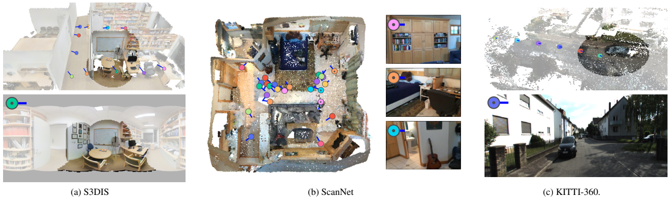
Figure 6. Datasets. Illustration of the sampling procedure for all considered datasets with point clouds alongside some of the available images. The 3D components of batches are constituted of spheres for (a) S3DIS, rooms for (b) ScanNet, and cylinders for (c) KITTI-360.
