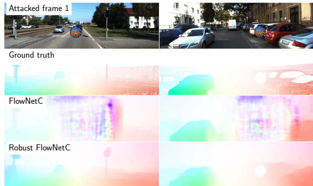
Figure 1. Overview. Physical patch-based adversarial attacks on optical flow can be avoided by minor architectural changes. First row: attacked first frame. Second row: ground truth optical flow. Third and fourth rows: the resulting optical flow estimates of FlowNetC [8] and our proposed Robust FlowNetC. FlowNetC is strongly affected by the adversarial patch, whereas Robust FlowNetC is barely affected. For the robust version we make simple design changes based on causes of the attack; see Section 6.
