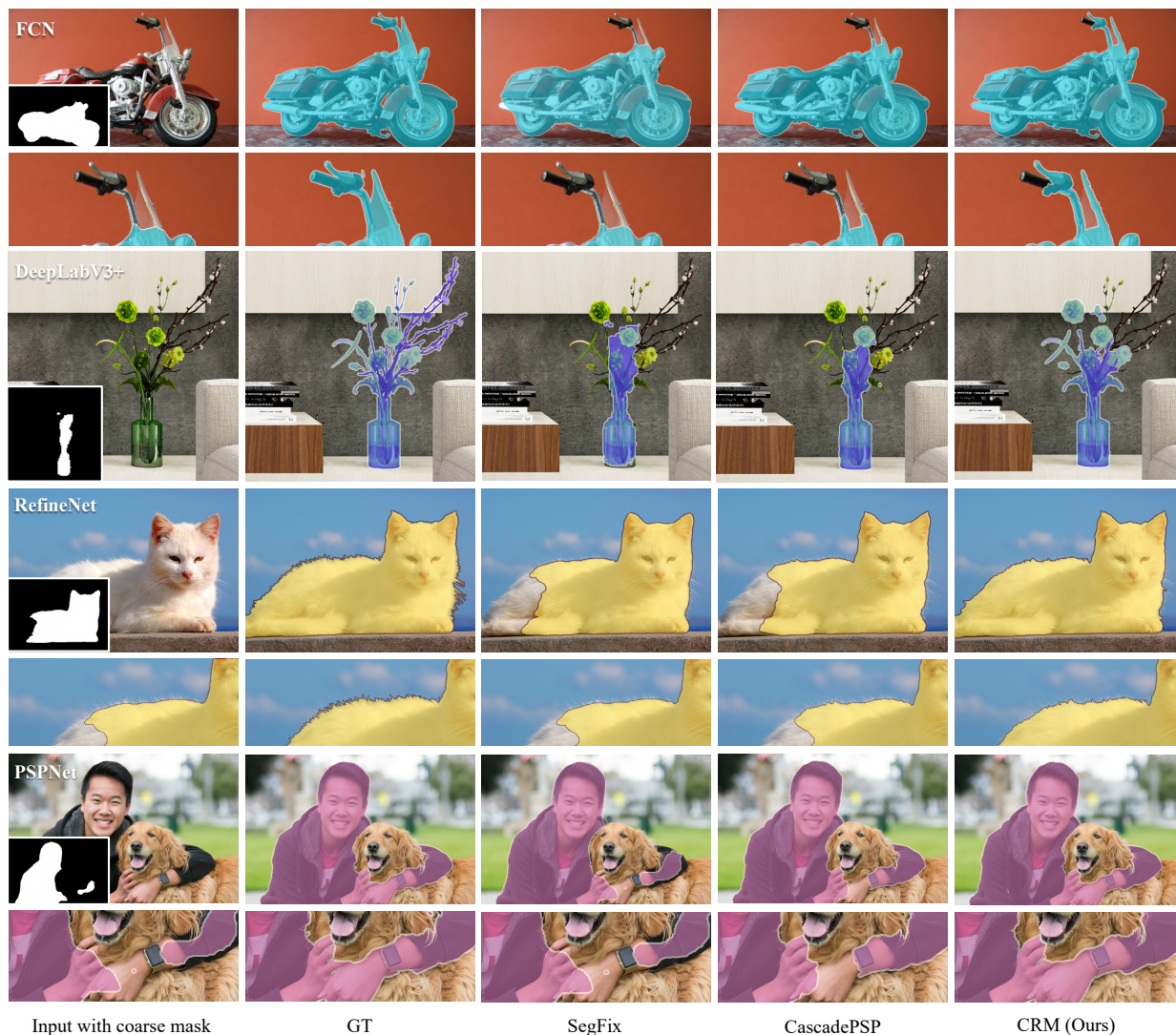
Figure 5. Qualitative comparison between Segfix, CascadePSP and CRM on the coarse mask from FCN, DeepLabV3+, RefineNet and PSPNet. The images are from BIG (2K ~ 6K). And the black-white mask in bottom left part of first column is the coarse mask.
