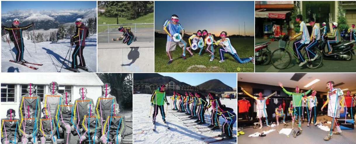
Figure 5. Visualization results of PETR. The first row and the second row show the visualization results on COCO val2017 and CrowdPose test set, respectively. PETR performs well on a wide range of poses, containing viewpoint change, occlusion, motion blur and crowded scene. Best viewed in color.
