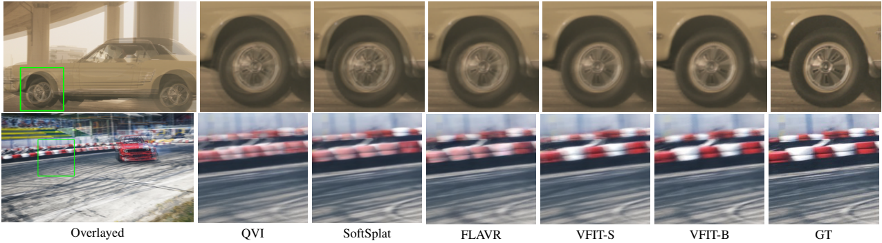
Figure 6. Overlap of interpolated frames and the corresponding ground truth, where a clearer overlapped image indicates a more accurate prediction. Note that for the second example, as the predictions of the baseline methods and the ground truth are not well aligned, the overlap of the red and white regions presents a blurry pink color.
