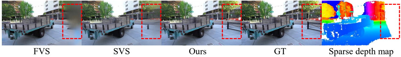
Figure 2. Visual comparisons with recent IBR methods on Tanks and Temples dataset. FVS [31] and SVS [32] will produce a blur in the area where the input sparse depth map misses, while our method can still synthesize a photorealistic result.
