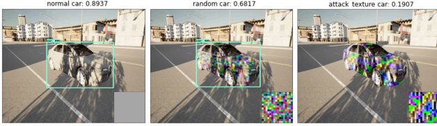
Figure 7. DTN texture rendering results with detection. From left to right: normal texture (detected as car), random texture (detected as car), attack texture (mis-detection). The car’s confidence score for attack textures is the lowest at 0.1907.
