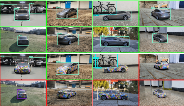
Figure 10. Real-world evaluation using two 3D-printed scaled models of Tesla Model 3. The upper rows are the standard model while the bottom rows are the attack model.
