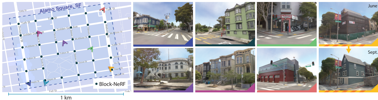
Figure 1. Block-NeRF is a method that enables large-scale scene reconstruction by representing the environment using multiple compact NeRFs that each fit into memory. At inference time, Block-NeRF seamlessly combines renderings of the relevant NeRFs for the given area. In this example, we reconstruct the Alamo Square neighborhood in San Francisco using data collected over 3 months. Block-NeRF can update individual blocks of the environment without retraining on the entire scene, as demonstrated by the construction on the right. Video results can be found on the project website waymo.com/research/block-nerf .
