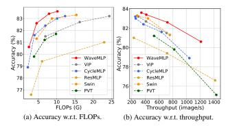
Figure 1. Performance comparison between the proposed Wave-MLP and existing architectures. Top-1 accuracies on ImageNet are reported.
