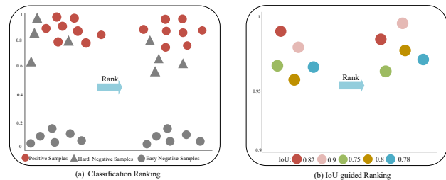
Figure 1. Illustration of the proposed two ranking losses. The classification loss enables positive samples to rank higher than hard negative samples, aiming to suppress the classification confidence of distractors. The IoU ranking loss aims to align classification with localization, i.e., that the samples with larger IoUs are expected to gain higher classification confidence scores.
