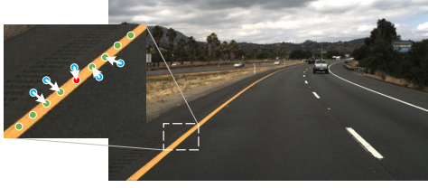
Figure 5. Illustration of the matching between predict points and their ground truth. The red dot is the observed keypoint. The blue dots are the predicted locations of adjacent keypoints. The green dots are the ground-truth locations of adjacent keypoints on the lane line.
