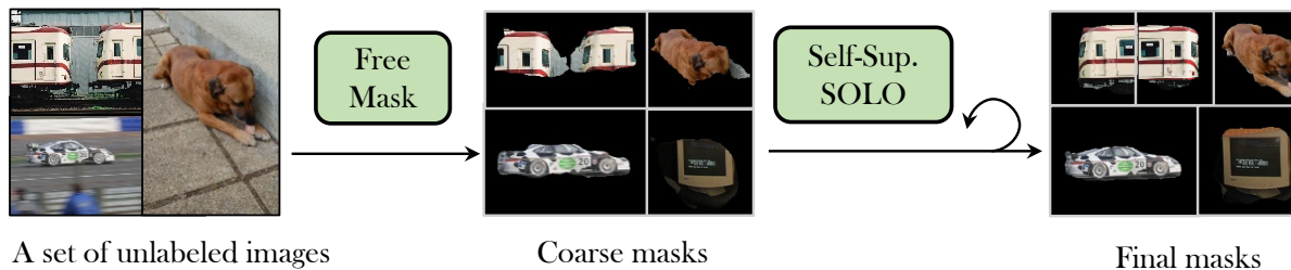
Figure 2. Overview of FreeSOLO. Unlabeled images are first input to Free Mask to generate coarse object masks. The segmentation masks as well as their associated semantic embeddings are used to train a SOLO-based instance segmentation model via weak supervision. We use self-training to improve object mask segmentation.
