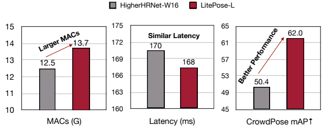
Figure 8. Compared with the multi-branch HigherHRNet-W16 [8], single-branch LitePose-L executes with higher parallelism. Therefore it achieves much better performance and similar latency on Qualcomm Snapdragon 855 with even higher MACs.
