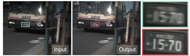
Figure 8. Generalization evaluation. We train our model on a certain RSGR camera and test it on another different RSGR camera, which has different exposure time, readout time, resolution, etc. Note that the scan direction is top-to-bottom ( \downarrow ).
