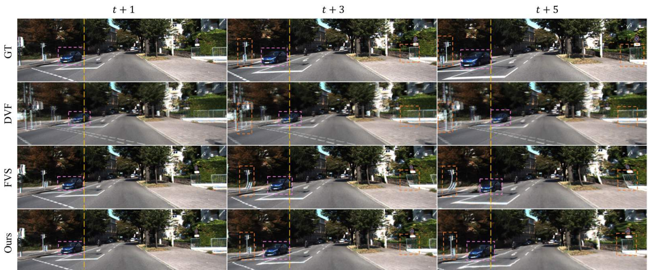
Figure 3. Multi-frame prediction comparison on KITTI. As the pink boxes show, DVF [20] fails to separate the motion of the blue car from the background and produces a “zooming-in” effect, which is the major motion exhibited in the dataset, caused by the forward movement of the running car. FVS [45] wrongly predicts the motion of the blue car at t + 3 and t + 5 , resulting in incorrect frame prediction results. Our model can correctly capture the motion of the blue car without external training.
