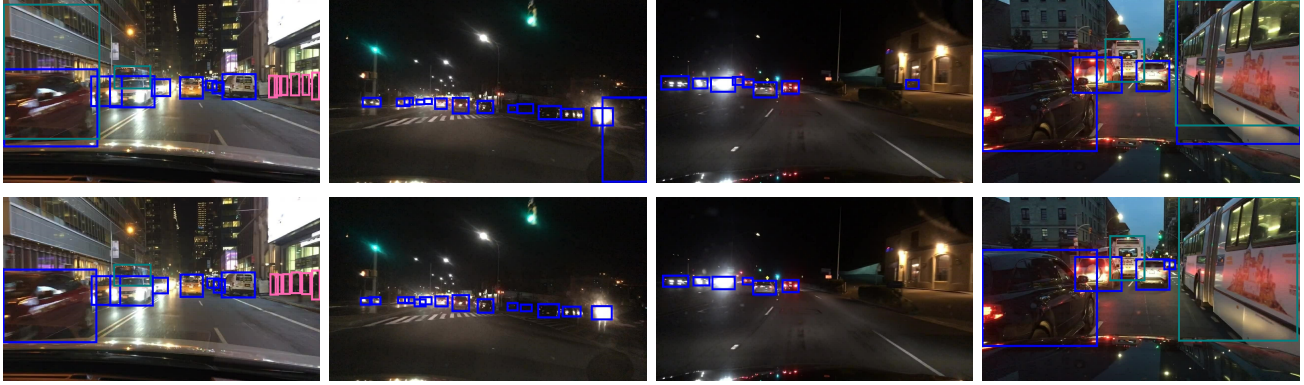
Figure 4. Detection results on the night-sunny scene. The first and second rows separately show the results from Faster R-CNN [33] and our method. We can see that compared with Faster R-CNN [33], our method could detect the objects accurately, e.g., the car, person, bus.
