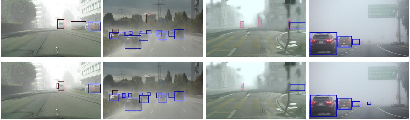
Figure 5. Detection results on the daytime-foggy scene. Compared with the results from Faster R-CNN [33] (as shown in the first row), our method (as shown in the second row) accurately detects objects in the foggy images, e.g., the car, person, truck.
