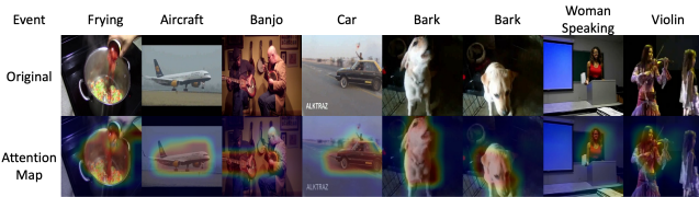
Figure 5. The qualitative results of our proposed cross-modal gated attention. The top row shows the event category, while the middle and bottom rows show the original video frames and visualization of the attention maps, respectively.
