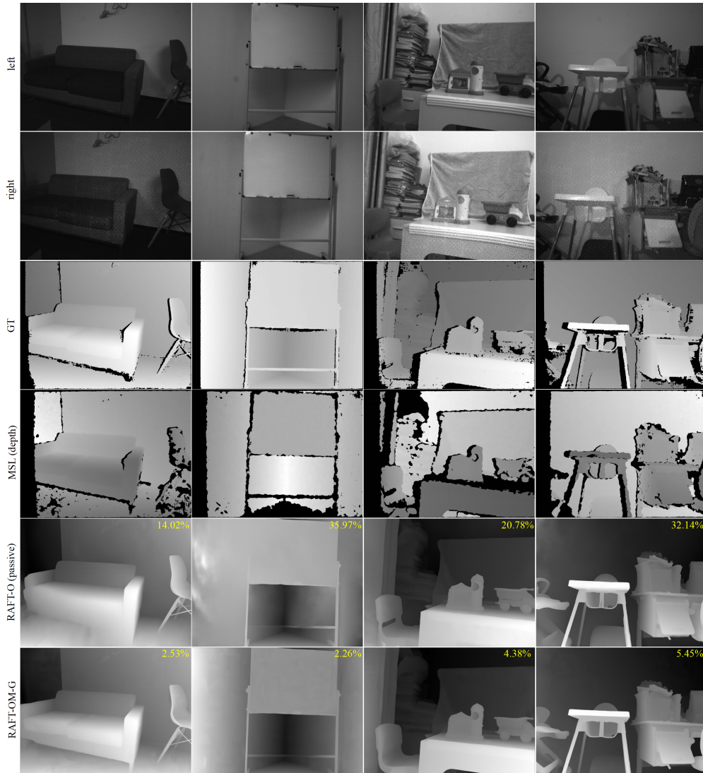
Figure 6. Comparisons on the real dataset. The first row shows the left images (The RGB images are converted to grayscale images before network prediction). The second row shows the right images with speckles (the passive right images are not shown), the third row is the ground truth disparity maps generated with the space-time stereo method [7, 46], the fourth row shows the depth images generated with the MSL subsystem, the fifth row shows the disparity maps of RAFT-O for the passive stereo images, and the last row shows the disparity maps of RAFT-OM-G, where the left image is passive and the right image is with speckles. In row 5 and row 6, Bad2.0 error is shown for each disparity map. The corresponding error maps are shown in the supplementary material.
