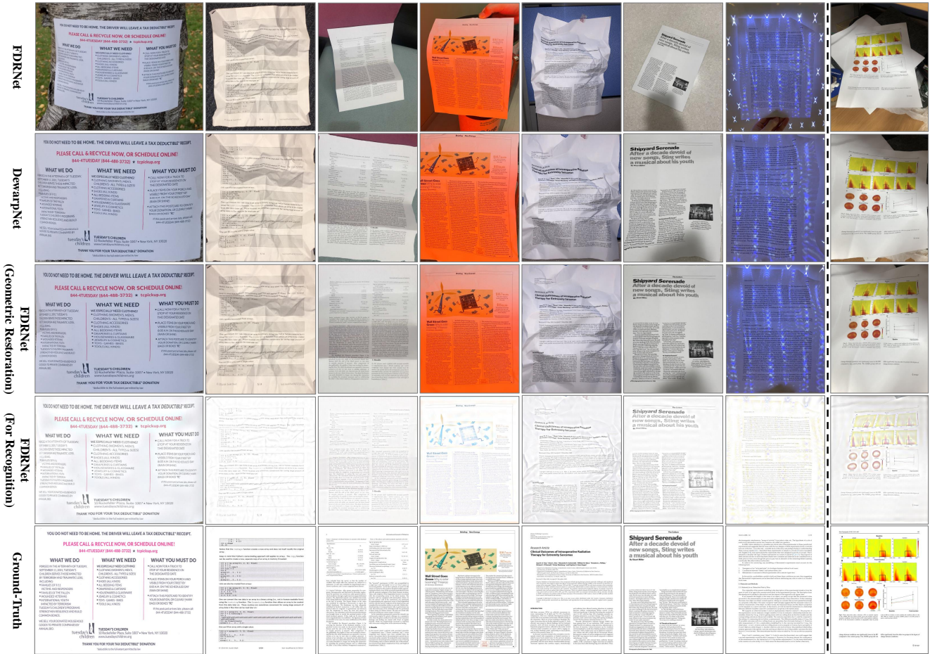
Figure 6. Illustration of document restoration by FDRNet and DewarpNet: For the sample images from DocUNet in columns 1-2 and WarpDoc in columns 3-8 in the first row, rows 2 and 3 show the dewarped images by using DewarpNet and FDRNet (dewarping on), respectively. Row 4 shows the appearance restoration by FDRNet which removes various appearance noises and improves document recognition greatly. FDRNet is robust to most geometric and photometric distortions but tends to get confused while document background has similar patterns as document regions as illustrated in the last sample.
