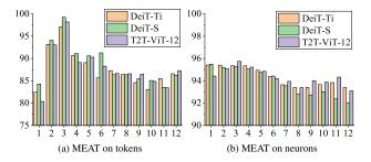
Figure 6. The activated rates of (a) image tokens in the MHSA block (b) neurons of the FFN block in each layer averaged on six new tasks of three ViTs using the MEAT attention mask.
