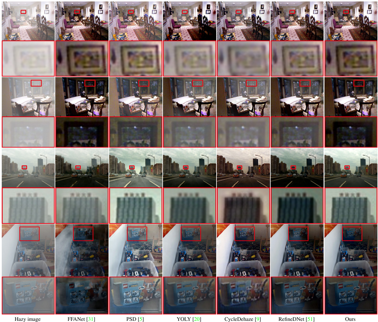
Figure 3. Visual comparison in haze removal on samples from the SOTS-indoor, SOTS-outdoor and I-HAZE dataset. FFANet only performs well on the first and second cases. All results of PSD, YOLY and CycleDehaze are hazy. The first, second and fourth cases of RefineDNet are hazy and the third case is over-dehazed. Our method dehazes well on all cases.
