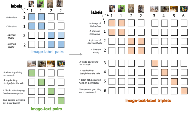
Figure 2. An illustration of covering image-label and image-text data in the image-text-label space. For image-label data, we associate a textual concept to each label, and the images and textual concepts are matched based on the annotated labels (blue tiles). For image-text data, each pair have unique label index, thus matched only at the diagonal entries (green tiles). On the right side, we can simply combine them as image-text-label triplets, and the red tiles means positive pairs while the blank tiles are negative pairs.
