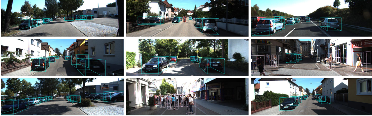
Figure 4. Qualitative results on KITTI val set. We visualize the detection results of 3D object detection from GUPNet [28] equipped with our dimension embedding module. The detected cars, pedestrians, and cyclists are represented with cyan, light pink, and red bounding boxes. (Best viewed in color.)
