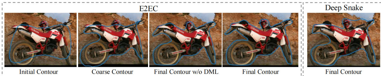
Figure 7. The prediction contours at different stages. The initial contour of E2EC fits the instance better than the octagonal initialization of Deep Snake. The quality of the coarse contour predicted by E2EC is comparable to the final contour predicted by Deep Snake. The final contour predicted by E2EC with DML perfectly outlines the motorcycle.
