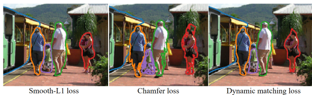
Figure 8. The prediction results supervised by different loss functions. Chamfer loss slightly improved the quality of boundary details but produced a serious jagged phenomenon (especially the red and purple instances). Dynamic matching loss heavily improved the quality of boundary details and did not cause any harm.
