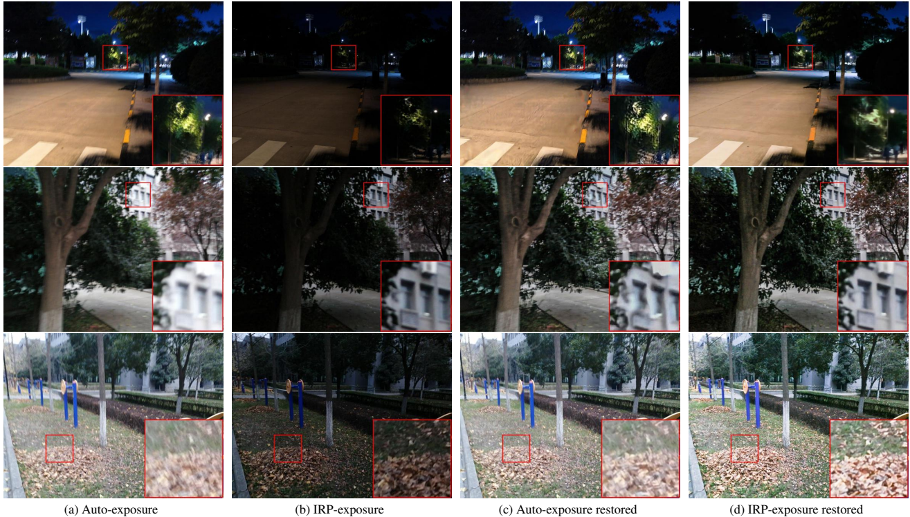
Figure 9. Comparison of IRP for optimizing exposure settings against conventional auto-exposure settings of camera.
