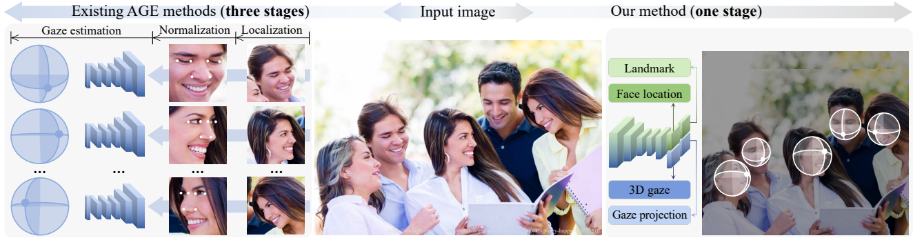
Figure 2. Comparison between existing appearance-based gaze estimation (AGE) methods and our method. AGE methods usually conduct localization, normalization, and gaze estimation for each face one by one. We present the first one-stage method to simultaneously estimate gaze directions for multiple people in one pass.
