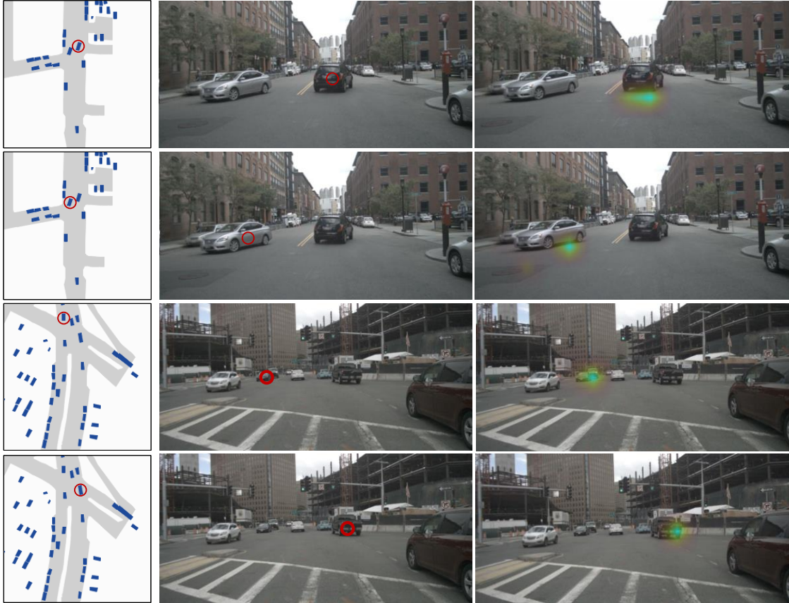
Figure 6. Visualization of cross-view attention. We compute attention from a point in map-view coordinates and visualize the corresponding attention values of the front camera view. Note how the network learns geometric correspondences through this attention mechanism.
