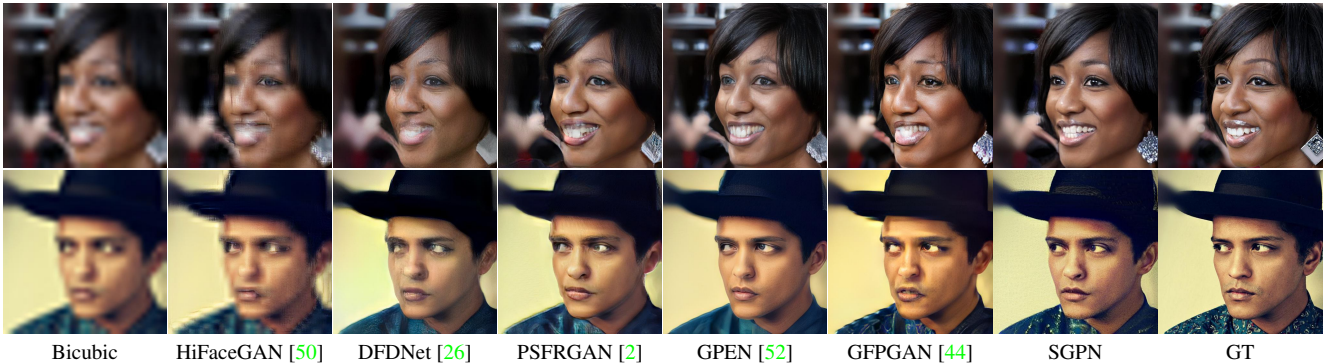
Figure 6. Visual comparison of Face Super-Resolution (FSR) . The ground truth HQ image is firstly downscaled and then upscaled to the original resolution with bicubic interpolation to synthesize LQ images. The scale factor is 16\times .
