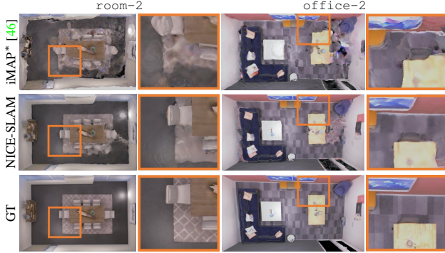
Figure 3. Reconstruction Results on the Replica Dataset [44]. iMAP* refers to our iMAP re-implementation.
