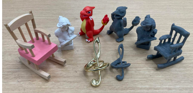
Figure 1. 3D printing of shape reconstructions. The proposed neural kaleidoscopic space sculpting can generate replicas of real objects with a range of shapes and reflectances. Reconstructed meshes are available on the project webpage [2].
