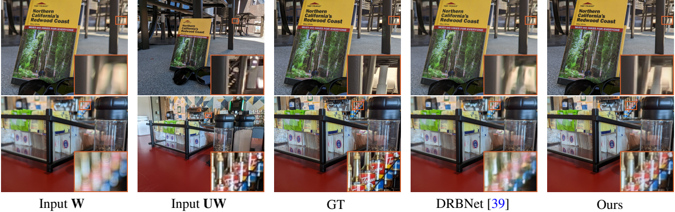
Figure 4. Defocus deblurring. We showcase the results of our method against SoTA single image defocus deblurring DRBNet [39]. Note that our method restores severely blurred regions in the background that single-image based methods often struggle with.
