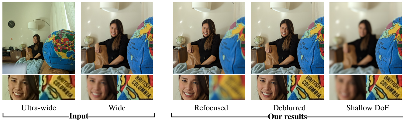
Figure 1. Post-capture depth-of-field (DoF) control from dual camera. (Left) Using photos captured from dual cameras with a wide field of view (FoV) and ultra-wide FoV, our method enables various DoF manipulations. (Right) We showcase our results of refocusing (changing the focal plane), deblurring (creating all-in-focus imagery), and synthesizing a shallower DoF (producing bokeh effects).
