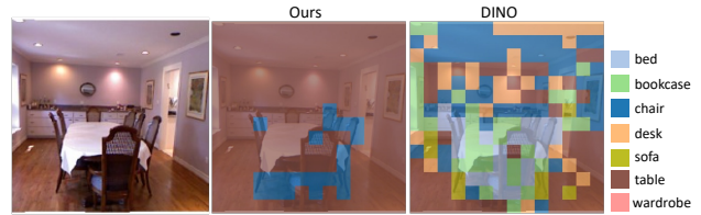
Figure 5. We compute the feature similarity between each patch in an unseen input image and the mean global feature of learned images in each category using models with a ViT-B backbone. Without fine-tuning , our model can identify the table and roughly localize patches associated with the chairs in the image by using the category of the most similar mean global feature of each patch.
