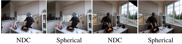
Figure 6. Synthesis Results at Extreme Views for NDC and Spherical Coordinates. Scenes represented in NDC are assumed to be bounded along x, y axes, whose boundaries are observable at extreme views (top-left and top-right corners), leading to incorrect geometries and artifacts. Using spherical coordinate, our HexPlane could seamlessly represent dynamic unbounded scenes.
