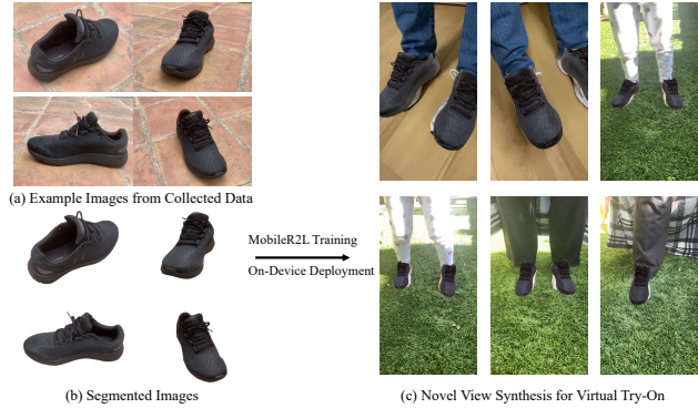
Figure 6. Virtual Try-On Application. From the collected images using a cellphone (a), we segment the foreground shoe (b) to train a MobileR2L model. We deploy the model on mobile devices, and users can directly try the shoe. The model renders images for novel views when users rotate the phone or change the foot positions (c).
