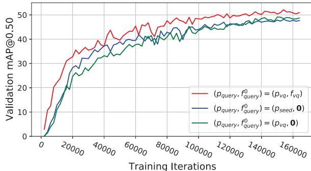
Figure 5. Vote query and convergence. We take out convergence study on a different combination of content feature f_{vq} and position p_{vq} in vote query. The baseline model (p_{query}, f_{query}^0) = (p_{seed}, \mathbf{0}) downgrades to 3DETR. Introducing p_{vq} boosts performance but decelerates training since FFN_{vote} requires time to converge, and f_{vq} accelerates training.
