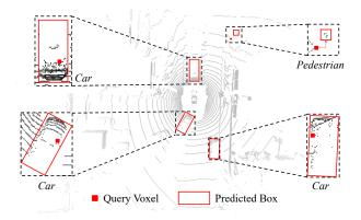
Figure 9. Visualization on the predicted boxes and their query voxels. For the *Car* objects, query voxels are inside and usually near the boundaries. For the pedestrian consisting of limited voxels, its query voxel is outside. More visualizations are in the appendix.
