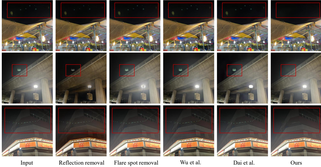
Figure 8. Visual comparison of different flare removal and reflection removal methods on real-world nighttime flare images.
