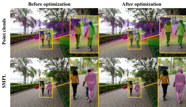
Figure 6. The comparison before (left) and after (right) extrinsic optimization by projecting the point clouds (upper) and SMPL (lower) are projected onto the image.
