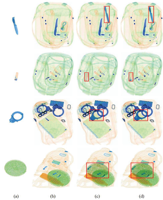
Figure 8. The generated images from the fusion module with only mask average pooling layer and our RWSC-Fusion module. From left to right are: (a) prohibited items; (b) original baggage image; (c) the synthesized images from the model with only mask average pooling layer; (d) the synthesized images from our model.
