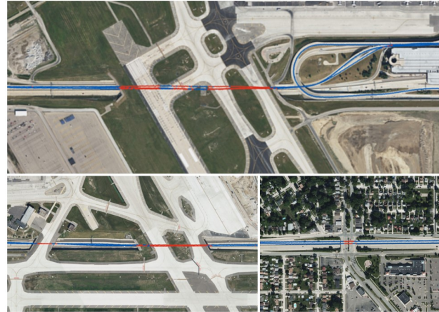
Figure 5. Examples of the data-pruning method on the Ford AV dataset [6]. Blue and red color represent kept and pruned frames in the trajectory. Map data: Bing Maps © 2022 TomTom, © Vexcel Imaging [1].
