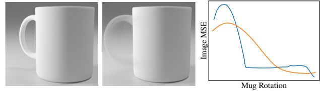
Figure 3. Optimizing the cup’s rotation in the hard (left, blue) and smooth (right, orange) setting (note the blurred handle). The image-space loss landscape is displayed on the right: blurring resolves the plateau.
