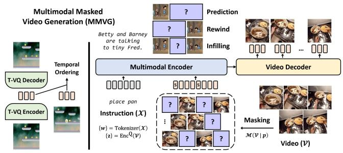
Figure 2. An overview of our Multimodal Masked Video Generation (MMVG). We present temporal-aware VQGAN (T-VQ) for discrete visual representation. MMVG considers the instruction  $\mathcal{X}$  and partial frames of the video  $\mathcal{V}$  from diverse time points through masking, learning to generate the complete  $\mathcal{V}$ . In this way, a single trained MMVG can perform all prediction, rewind, and infilling tasks.
