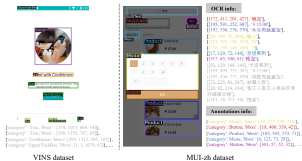
Figure 1. Two MUI samples from VINS and MUI-zh dataset. Compared to VINS, we additionally obtain the OCR descriptions as supplemental information in MUI-zh. Moreover, we further link OCR descriptions and element annotations with the same color.
