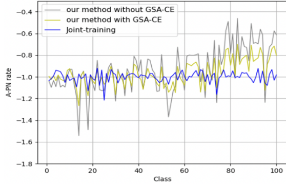
Figure 3. The gradient rate after the model has learned all classes of CIFAR100. A-PN is the gradient rate. The memory buffer size is 1000. Joint training means the model learns all classes together as one task in one epoch.
