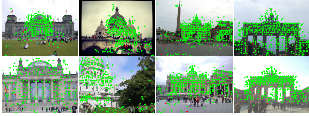
Figure 5. Qualitative results on the YFCC100M (the first two columns) and MegaDepth datasets (the last two columns). The images in each column form a pair for image matching. Green and red dots denote correct and incorrect matches respectively. (The epipolar error threshold is 5 \times 10^{-4} ).
